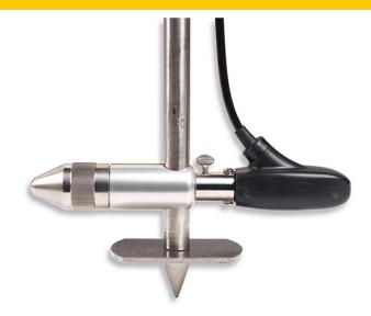
Handheld electromagnetic water flow meter with automatic discharge calculation
